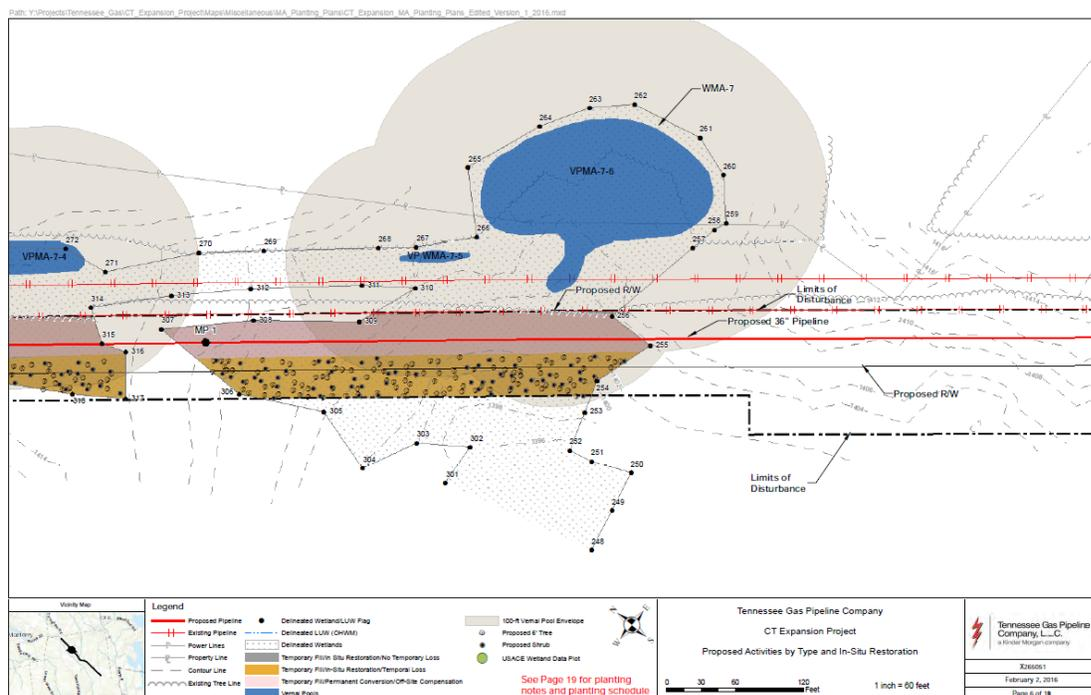
Figure 42. Alignment and wetland mitigation plan for a section of an approved natural gas pipeline in New England. Image courtesy of FERC.
