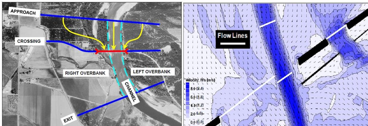
Figure 60. 1D and 2D hydraulic modeling for bridge design. Images courtesy of Federal Highway Administration.
