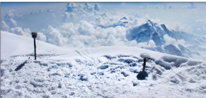
The survey gear on the summit: NetR9's Zephyr-2 antenna (R) and R10 (L).
