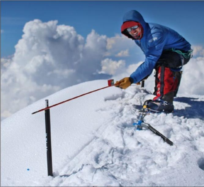
Udi Karriere levels the two range poles to ensure both the R9 and R10 are at the same elevation.
