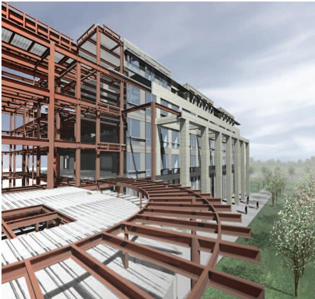
▲ BIM enabled PSA-Dewberry to create a proof-of-concept model to validate the systems and components for each discipline
