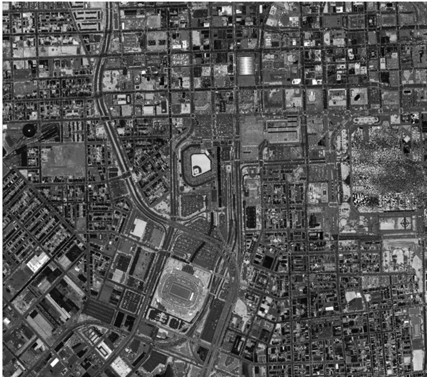
Normally, IFSAR clearly delineates water areas, but LIDAR does not, as shown here.
