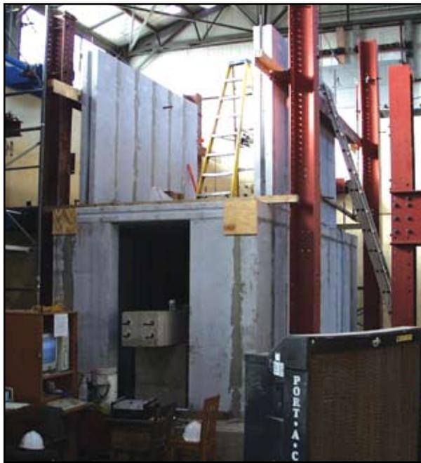
*Building two-story assemblage for testing specimen at University of Texas at Austin. Courtesy of UT Austin.*
