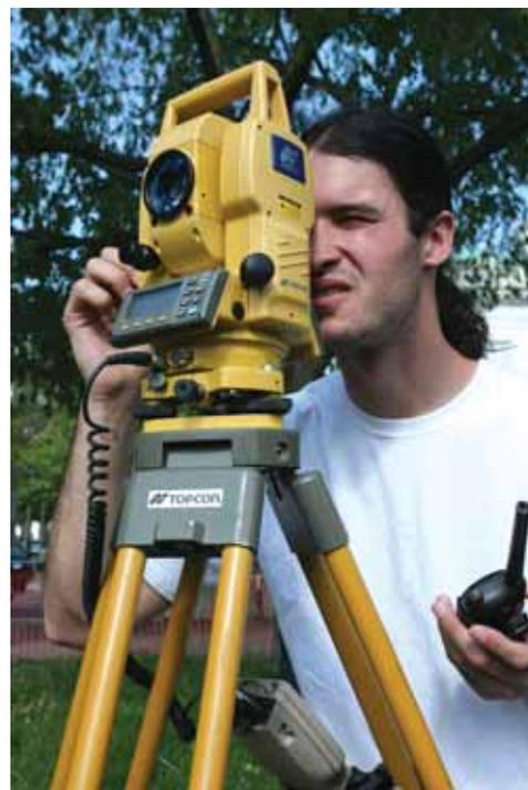
▲ Kris Noel, a surveyor with Dewberry, takes measurements for use in a flood insurance rate map. FEMA requires that data from technologies such as LiDAR be supplemented with traditional survey techniques.
