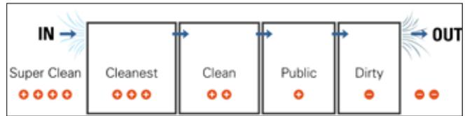
FIGURE 4. Moving air via pressure differentials.
